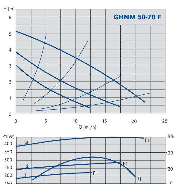
**Three speeds twin circulation pumps with flanges - mono-phases voltage
